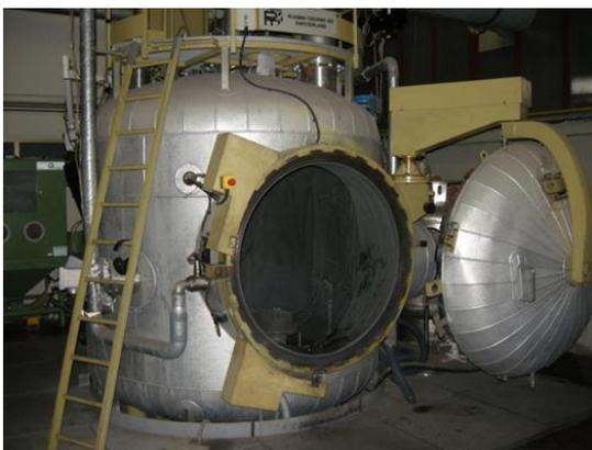
Fig. 1: Controlled atmosphere Plasma Spray equipment
