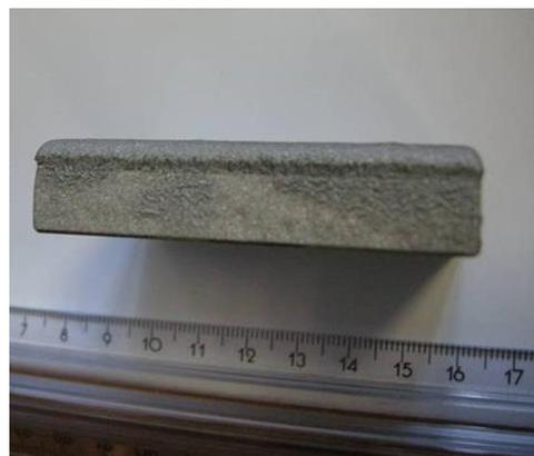
Fig. 2: Example of thick tungsten coating
