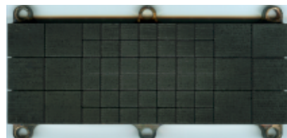
Carbon fibre composite (CFC) structure used in fusion for wall protection from high heat flux (Source: S. Peschany)
