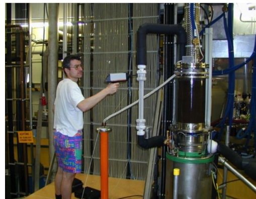
Application of Axial Potential Separator in Fusion Domain (Source: S. Fink: Cryogenic insulation break", KIT, October 31st, 2014)
