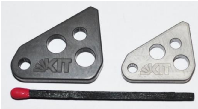
Fig. 1: Langmuir probes for the WEST project produced via PIM @ KIT
