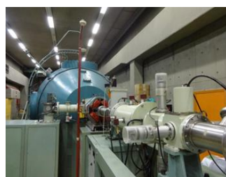
Depth profile of deposited elements in tungsten JET divertor after plasma exposure (left) employing nuclear reaction analysis with deuterium ions ( 2 H) at the TANDEM accelerator at NCSR “Demokritos” (right)
