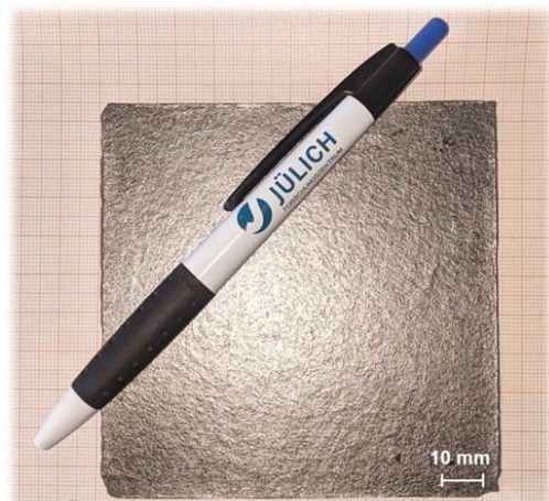
Figure 4: A large-scale bulk SMART alloy sample sintered using the industrial FAST facility.
