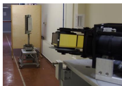
Short range high resolution (radiation resistant prototype submillimetric resolution up to 10 meters )
