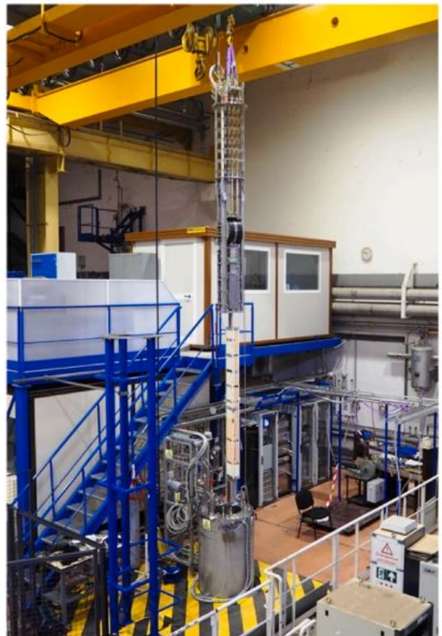
Test assembly insertion inside the cryostat
